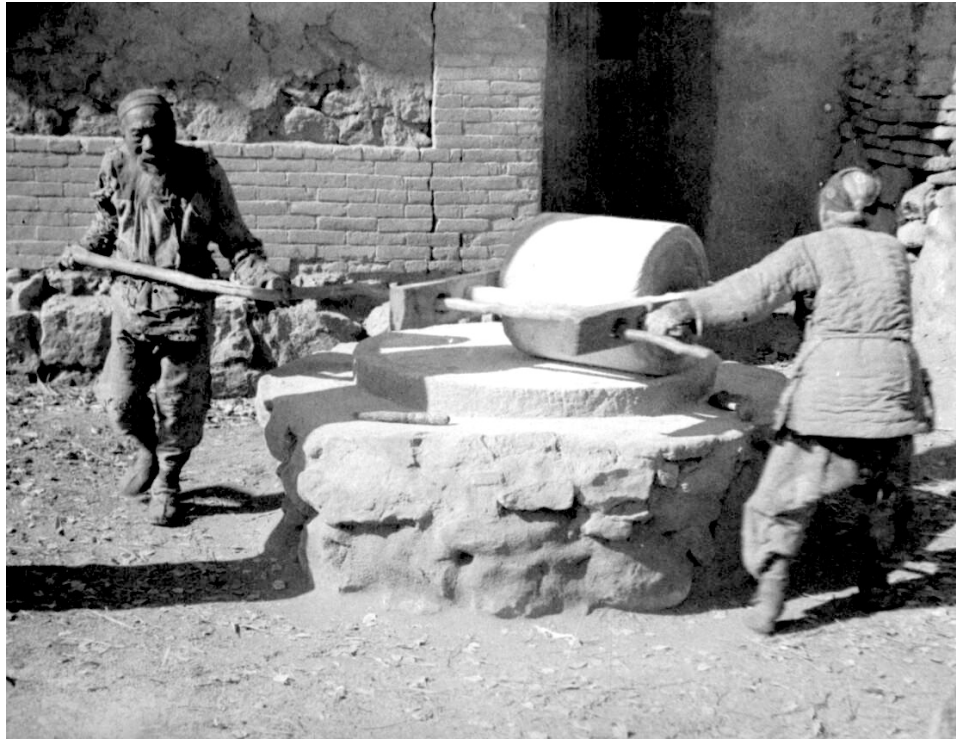
Figure 11.8: Old couple grinding grain. Note that the roller is not tapered. Thus it skids on the lower stone as it is turned and grinds as well as crushes the grain. There are two whisk brooms on the mill mount that are used to sweep any partly ground grain back under the roller.
